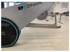
6. Attach the front leg to the bar using the remaining two bolts and nuts to fully suspend the machine. This can be made easier if you have someone else to hold the bars up for you. Insert the black plastic plugs over the boltheads as before.
