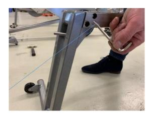
7. Attach the footplates to the machine by sliding the two rods through the footplates and the main machine assembly. Secure the rods with the stainless steel end bolts. The footplates are attached with the strap buckle on the outsides.
