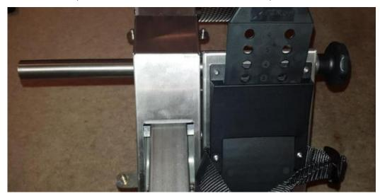
8. Remove the flywheel locking bolt (red bolt) to free the handle.
