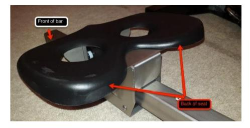
4. Carefully align the front of the bar with the bearings inside the flywheel assembly at the footplate end and slide the bar into the machine. Ensure that the locking pin is in the green, unlocked position before doing this.
